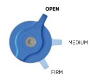
The **3-position lever** is useful to make on-the-fly adjustments to control fork performance under significant changes in terrain, and is intended to be adjusted throughout the ride.
